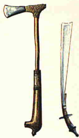
BLACKSMITHS FROM THE PENINSULA (FACING PAGE) AND SARAWAK (THIS PAGE) FASHION HOT METAL INTO BLADES. TOOLS LIKE THE ADZE AND PARANG (ABOVE) FROM EAST MALAYSIA ARE MADE IN THIS WAY
