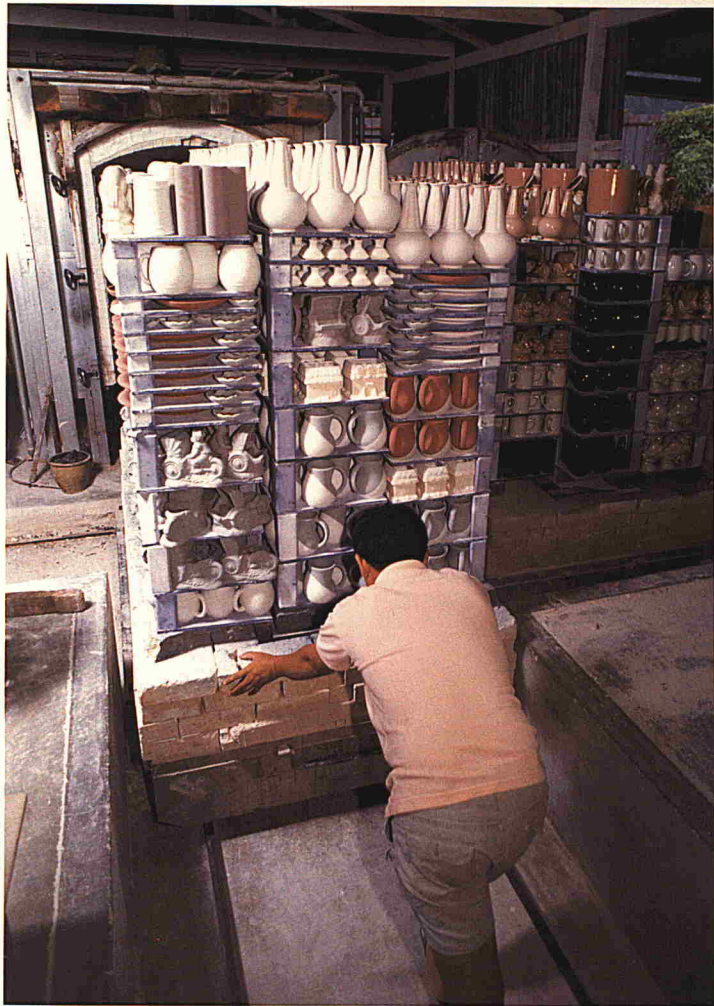
FACING PAGE, TOP: A STACK OF FLOWER POTS MADE USING A JIGGER TYPE OF MACHINE. IN CHINESE DRAGON KILN POTTERIES FROM THE IPOH DISTRICT. A DRAGON KILN MAY BE UP TO 45M LONG, WITH INTERNAL DIMENSIONS OF TWO METRES HIGH AND TWO METRES WIDE. THESE DRAGON KILNS WERE FIRST INTRODUCED INTO THE COUNTRY TO MAKE THE RUBBER CUPS USED BY RUBBER PLANTATIONS. BOTTOM PICTURE SHOWS A DRAGON KILN BUTTRESSED WITH A THICK WALL OF BRICKS AS SUPPORT. A DOORWAY FOR LOADING POTS CAN BE SEEN IN THE MIDDLE THIS PAGE. A KILN-CAR OF POTTERY IS PUSHED INTO A SHUTTLE KILN FOR FIRING. MORE INDUSTRIAL KILNS OF THIS TYPE ARE NOW BEING INTRODUCED TO MEET THE GROWING DEMAND FOR HIGH-END CERAMIC WARE.
